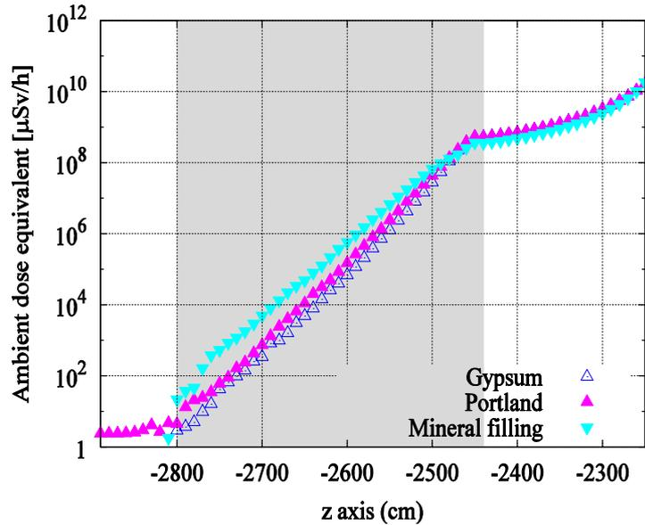
**FIGURE 5.** Comparison of the attenuation efficiency of concrete and sandwich-like structure with gypsum or blast furnace waste as filling. The irradiated target is made of SiC. The z axis represents the direction of the secondary particles (mainly neutrons) coming from the interaction of the proton beam with the uranium carbide target (from the right to the left). The white background in the picture indicates air while the grey background indicates the wall.
