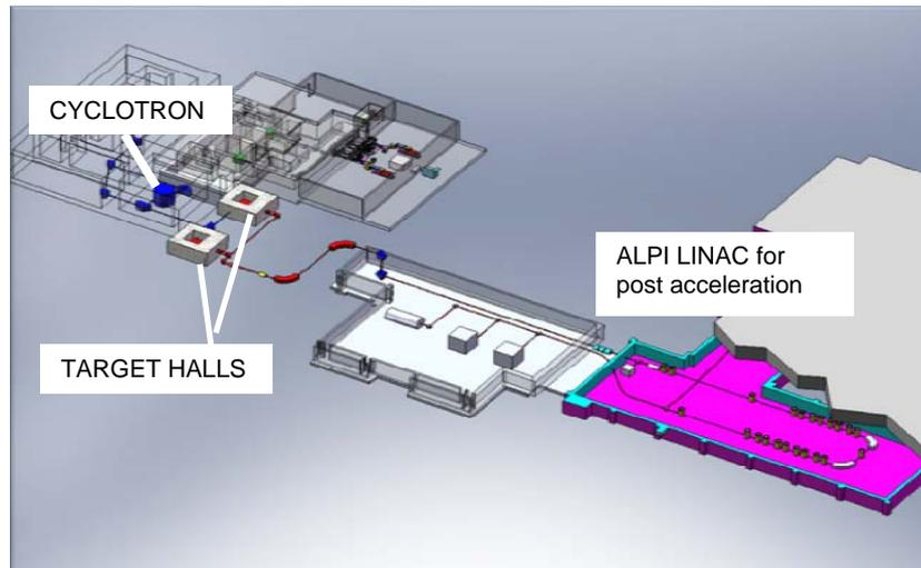
**FIGURE 1.** SPES layout: the ALPI linac already exists while the cyclotron vault and the target halls have to be built yet.
