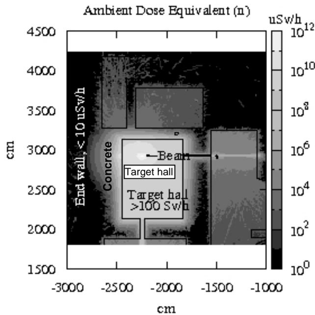
**FIGURE 3.** Ambient dose equivalent rate ( $\mu\text{Sv/h}$ ) due to neutrons in the target hall and adjacent rooms. The z axis represents the direction of the beam (from the right to the left) and the x axis represents the RIB extraction direction
