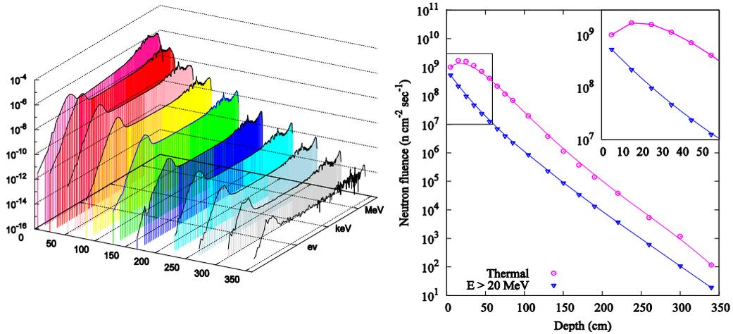
**FIGURE 2.** Left: neutron energy spectrum as a function of depth in concrete ( $\text{n/cm}^2/\text{proton on target}$ ). Right: thermal ( $E < 1 \text{ eV}$ ) and high energy neutrons ( $E > 20 \text{ MeV}$ ) as a function of depth in concrete.
