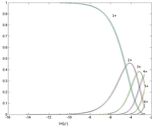
Figure 4: Ion charge state time evolution for Xe. The lower curves refer to an electron beam with hollow radius of 30% with respect to e-beam radius (upper curves).
