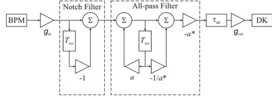
Figure 4: Block diagram of feedback loop with the notch and all-pass filters.
