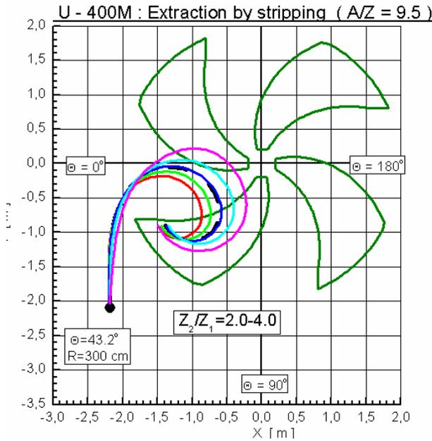
Figure 3: Trajectories of the low energy ion beams extracted from U400M cyclotron by method 1.
