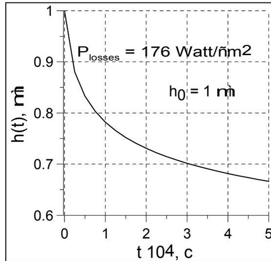
Figure 10: Evolutions of the carbon foil thickness
