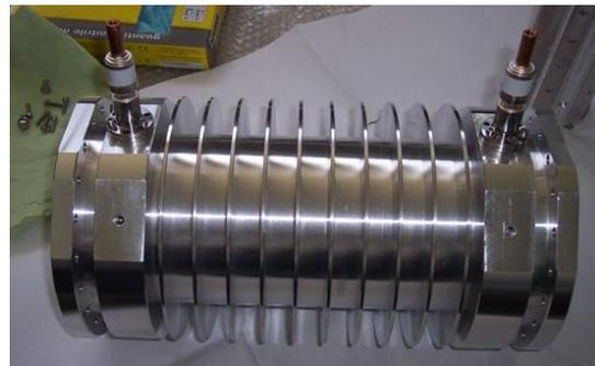
Figure 5: Chopper Faraday cup body, that is the vacuum chamber section just behind the Chopper magnet. Thin metallic tabs are machined on the body itself, in order to enhance heat evacuation by air-convection.
