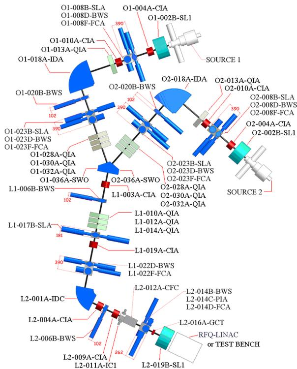
Figure 2: LEBT line layout. Sketch of magnets and beam diagnostics tanks, from the sources to the test bench installed at the end of the LEBT line. Legend: SLA= Slit monitor, FCA= Faraday Cup, BWS= Wire Scanner, CFC= Chopper Faraday Cup, GCT= AC- Current Transformer, PIA= Wires Harp, CIA= corrector, QIA= quadrupole, SL1= solenoid, SWO=switching magnet, IDA= 90° dipole, IDC=75° dipole, IC1 = Chopper dipole.
