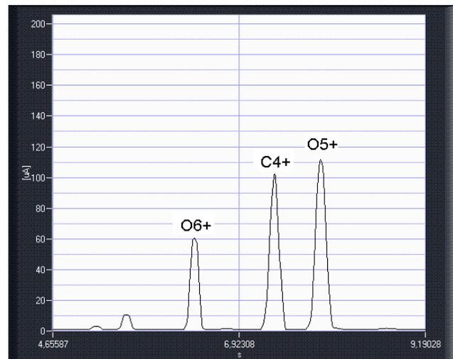
Figure 3: Source spectrum measured at the O2-023-FCA Faraday Cup, while ramping the O2-sector spectrometer from 30A to 60A. O2-023-SLA plates are positioned as follows: top and bottom plates fully out from beam path, left plate at -5 mm and right plate at +5 mm with respect to the vacuum chamber centre. One can notice the  $C^{4+}$  peak surrounded by other species peaks.
