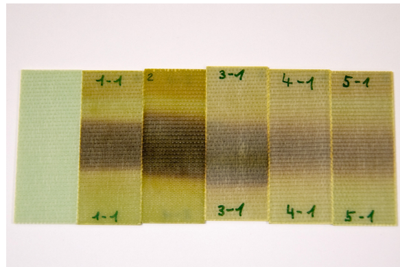
Figure 7: Dependence of the received dose on the segment: "1-1" is the first G11 plate of samples S11 in Segment 1, "2" – first plate of S11 in Segment 2, and "3-1", "4-1", "5-1" – first plates of S11 in Segments 3,4,5.
