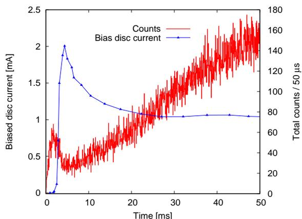
Figure 4: Comparison of time-resolved biased disc current and bremsstrahlung count rate. Rf pulse pattern: 50 ms on / 500 ms off.
