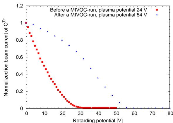
Figure 2: Normalized “plasma potential curves” with a clean aluminium plasma chamber and under heavy carbon contamination due to a MIVOC-run.
