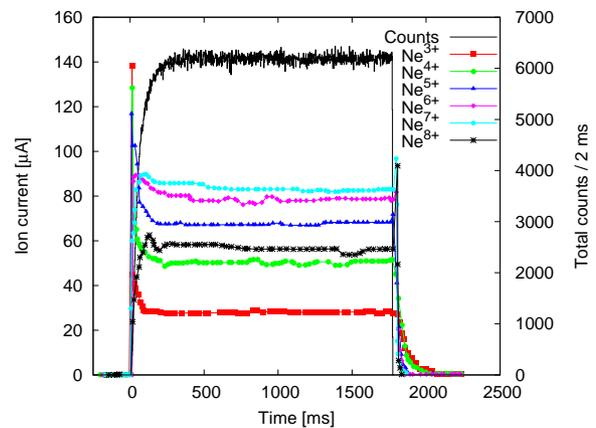
Figure 3a: Time-resolved ion currents of neon and corresponding bremsstrahlung count rate.
