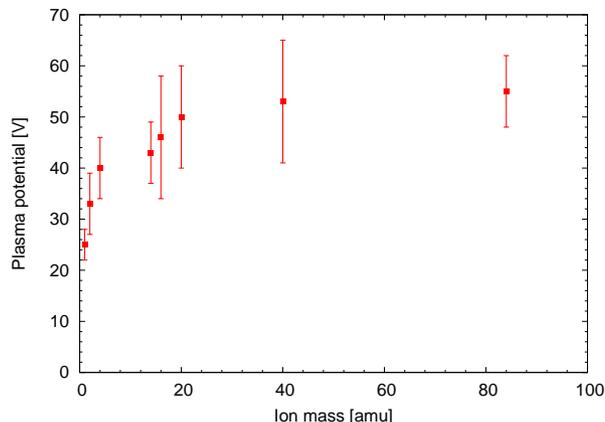
Figure 1: Plasma potential of the JYFL 6.4 GHz ECRIS as a function of ion mass. Vertical range corresponds to the variation of ion source parameters within typical limits.
