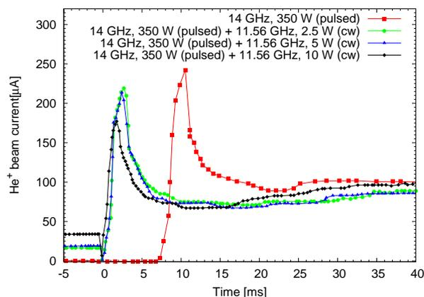
Figure 5a: Time-resolved ion beam currents of  $\text{He}^+$  with and without seed electrons provided by TWTA.
