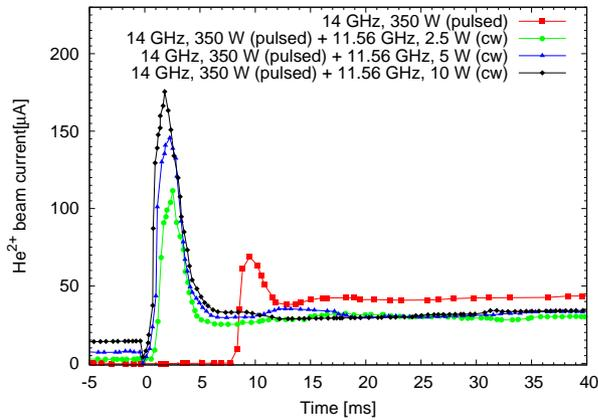
Figure 5b: Time-resolved ion beam currents of  $\text{He}^{2+}$  with and without seed electrons provided by TWTA.
