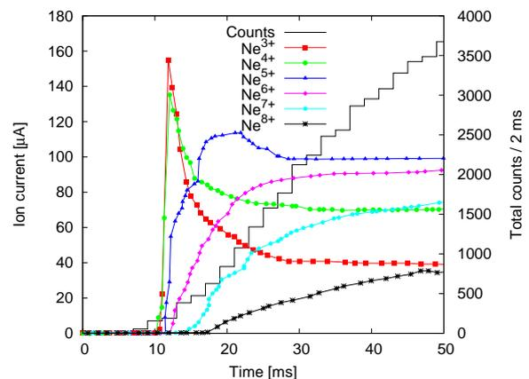
Figure 3b: Time-resolved ion currents of neon and corresponding bremsstrahlung count rate in the beginning of the rf pulse.
