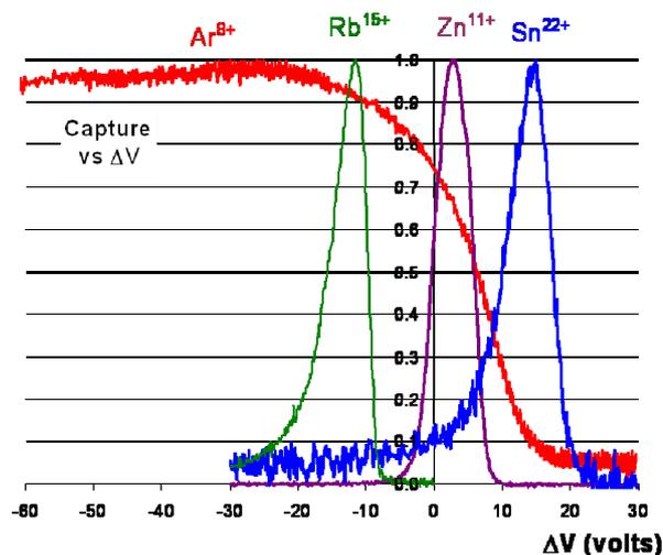
Figure 2: Normalized  $\Delta V$  plots for various elements and 1+ sources.
