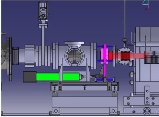
Figure 3: Mechanical setup for the movement of the grounded tube.
