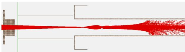
Figure 5: 1+ trajectories without decelerating tube.
