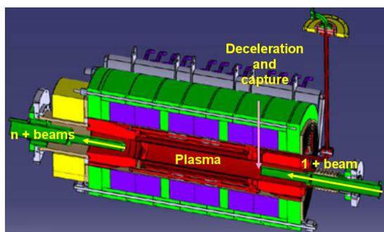
Figure 1: Cut view of the PHOENIX ECR charge breeder.
