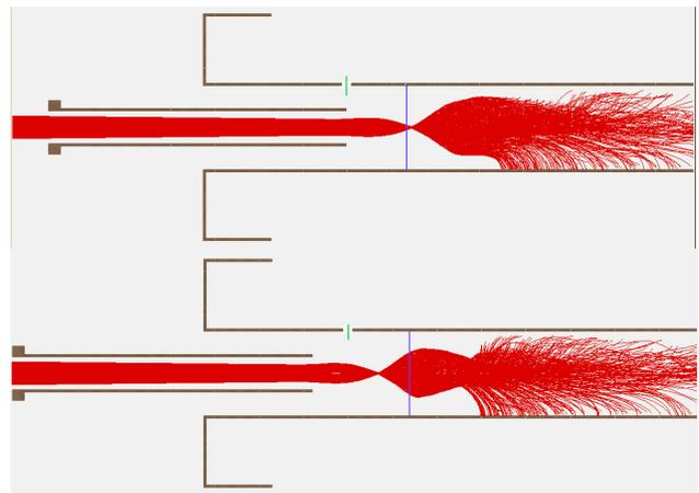
Figure 4:  $1+$  trajectories during deceleration for two positions of the grounded tube.
