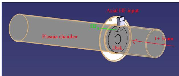
Figure 5: HF and 1+ beam injections in the plasma chamber without decelerating tube.
