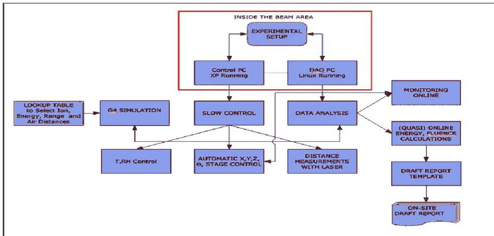
Figure 2: The configuration of DAQ and control PCs (inside the beam area) and laptop in control room. The tasks carried out by each computer are also shown.
