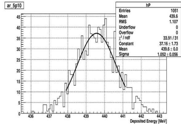
Figure 4: For <sup>40</sup>Ar beam at 10 cm air thickness (A2) Distribution of energy deposited in silicon simulated by Geant4.
