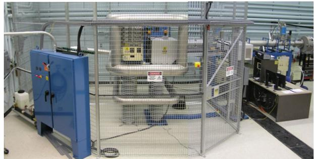
Figure 2: 400-kV ion implanter.
