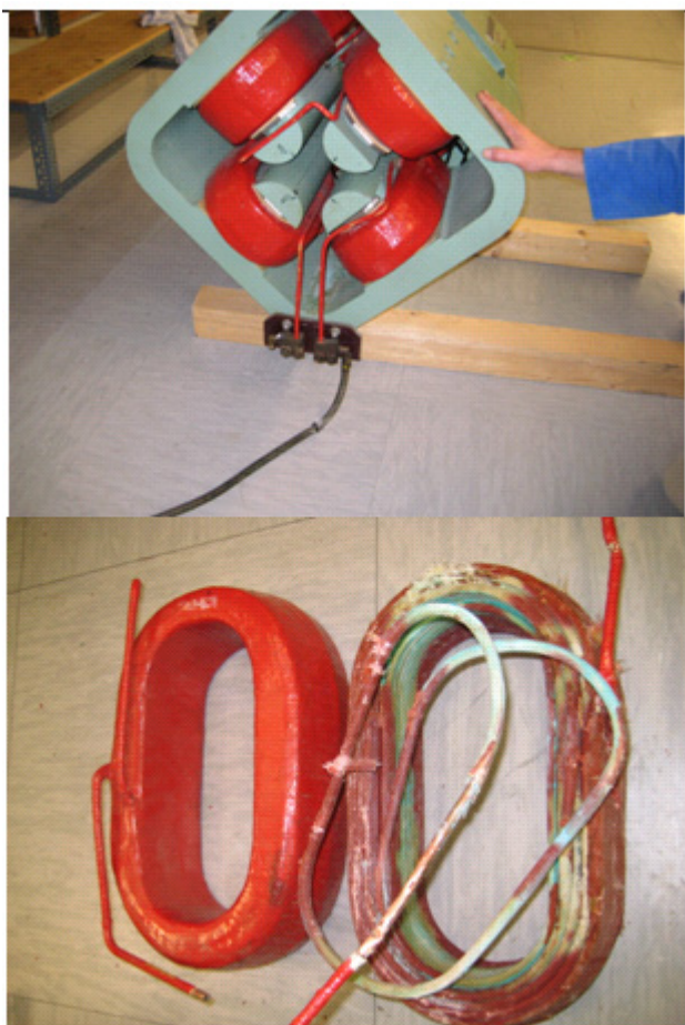
Figure 4 : Quadrupole lens at the exit of the accelerator and the defective coil.
