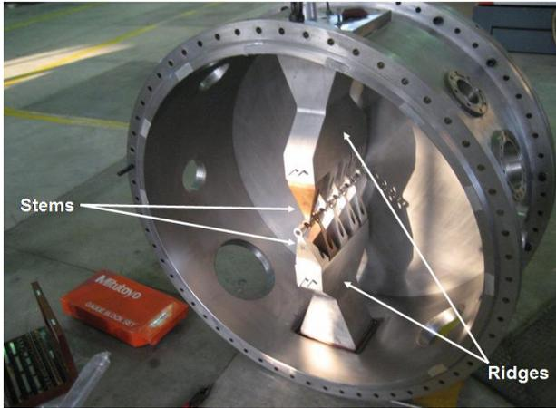
Figure 5: Prototype DTL cavity with stems and ridges.
