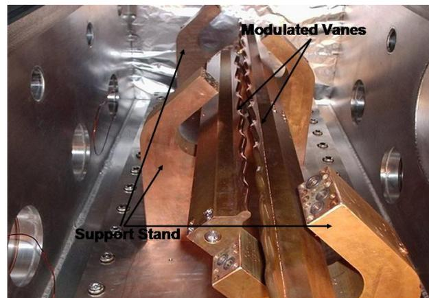
Figure 4: Modulated vanes of RFQ in the chamber.
