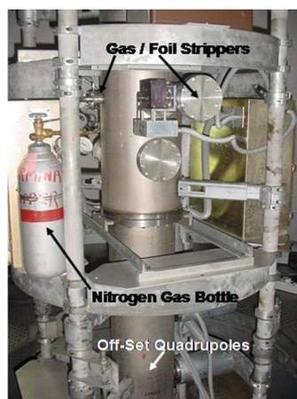
Figure 1: Off-set quadrupoles after strippers in terminal.
