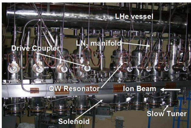
Figure 2: First linac having eight QWRs and superconducting solenoid.
