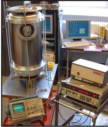
Figure 2: Parts clamped in *birdcage* for a frequency measurement.
