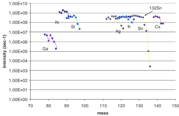
Figure 1: Expected on-target intensities calculated considering emission, ionization and acceleration efficiencies (see text) for different isotopes.
