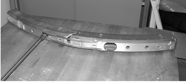
Figure 2: Water cooling circuit assembled in the rear part of the deflector housing.
