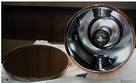
Figure 2: An upgraded medium  $\beta$  cavity with its tuning plate.
