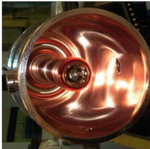
Figure 1: A high  $\beta$  cavity before being sputtered.
